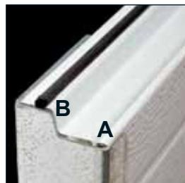
A continuous thermal break (A), prevents heat-loss by eliminating metal-to-metal contact between inside and outside door surfaces. An air seal (B) blocks airflow between sections.
