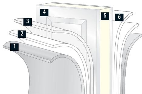
The 1-3/8" thick door sections of Buildmark STS™ are made from two layers of strong, rust-resistant 25-gauge galvanized steel and are coated with a baked-on polyester paint finish for long life.
